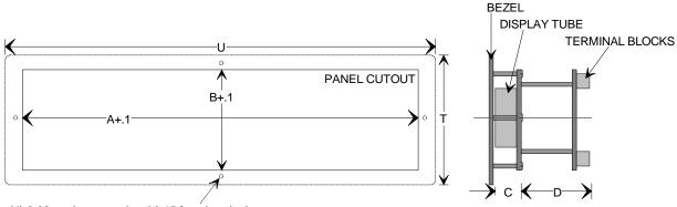
(4) 6-32 studs centered and 0.15 from bezel edge. Mounting studs of bezel fit through clearance holes drilled in panel.
