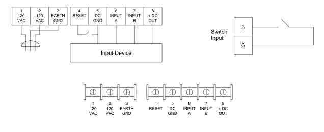
SAFETY GROUND : On AC power units, use a 3 wire grounded power terminal with the earth ground tied to terminal 3.
