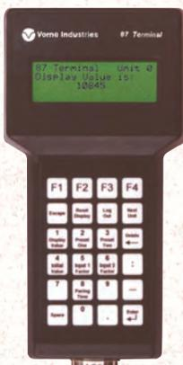
Want on line access to your 87 series displays? Our hand held terminal allows you to view and modify presets, scale factors and more for individual or networked 87 series displays. Power is provided by the 87 series display. The standard 24 key keypad and 4 line by 20 character LCD display help make this terminal extra easy to use.
