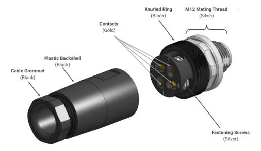
To wire a connector, remove the plastic backshell and thread wires through to contacts. Follow the specified Contact Pairings below and replace backshell. Screw the grommet at the back of the M12 connector until the wire is compressed.
